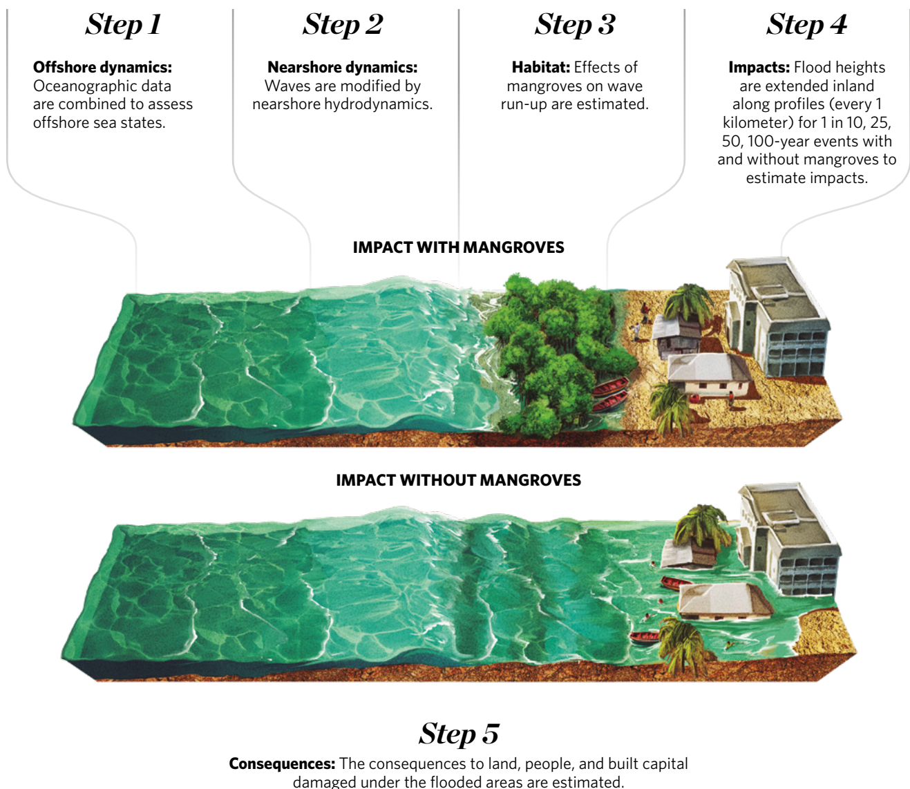
Figure 2: Key steps and data for estimating the flood protection benefits provided by mangroves (adapted from Beck et al. 2019). © Puntoaparte Editores.
